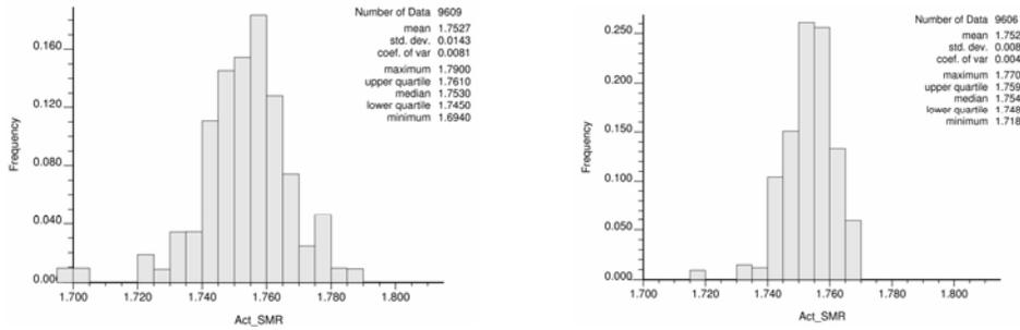
**Figure 19:** Histograms showing two different sets of furnace feed. The histogram on the left shows the variability in the furnace feed for the low selectivity grade control and the histogram on the right shows the variability for the base case grade control. The low selectivity case has almost twice the variability compared to the base grade control case.
