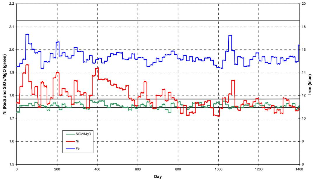
**Figure 21:** Furnace feed for the low selectivity samples, base case stockpiles, and base case stacker piles.
