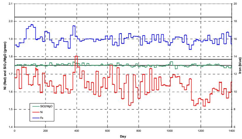
**Figure 18:** Simulated furnace for the base case. The green line represents the SMR, the red line is the nickel grade, and the blue line is the iron grade.
