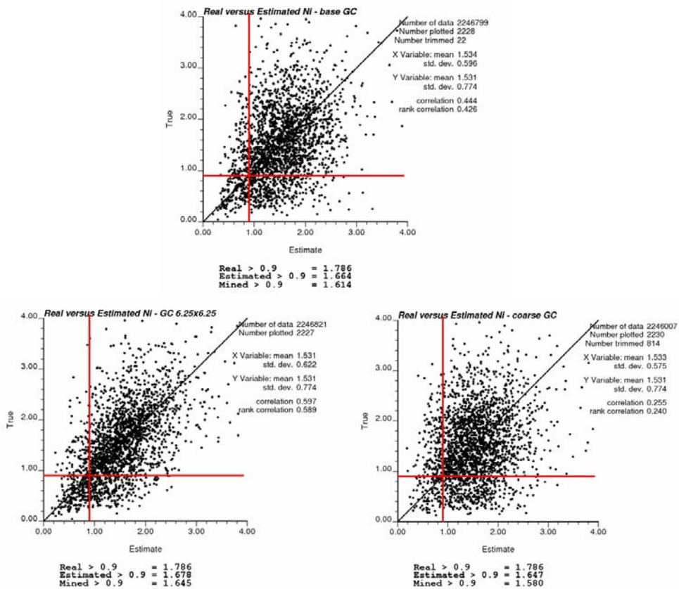
**Figure 24:** Check for the impact that the grade control drilling has on the nickel grade. The base case grade control drilling is on the top, the close spaced drilling is in the lower left and the coarse drilling is in the lower right.
