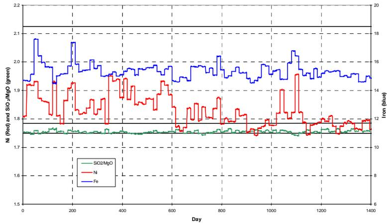
**Figure 23:** Furnace feed for the high selectivity samples, base case stockpiles, and base case stacker piles.
